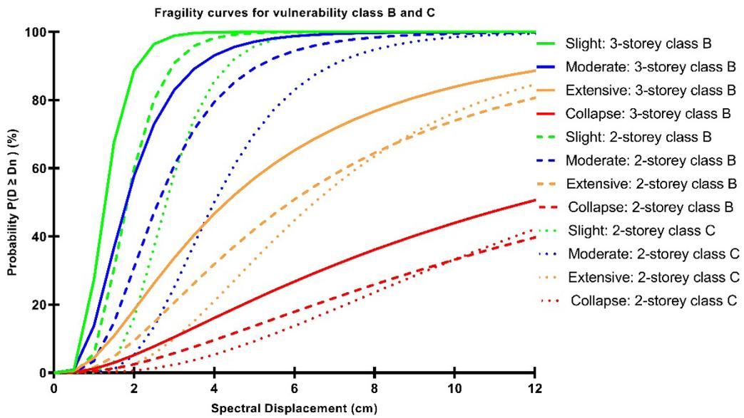
Figure 8b. Fragility curves for the selected seismic classes B and C.
