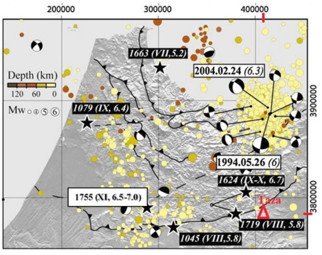
Figure 1. Summary map of instrumental and historical seismic activity affecting the city of Taza. The map shows the focal mechanisms of the main instrumental earthquakes. The red triangle on the map indicates the position of the city of Taza (modified after Poujol *et al.* 2014).
