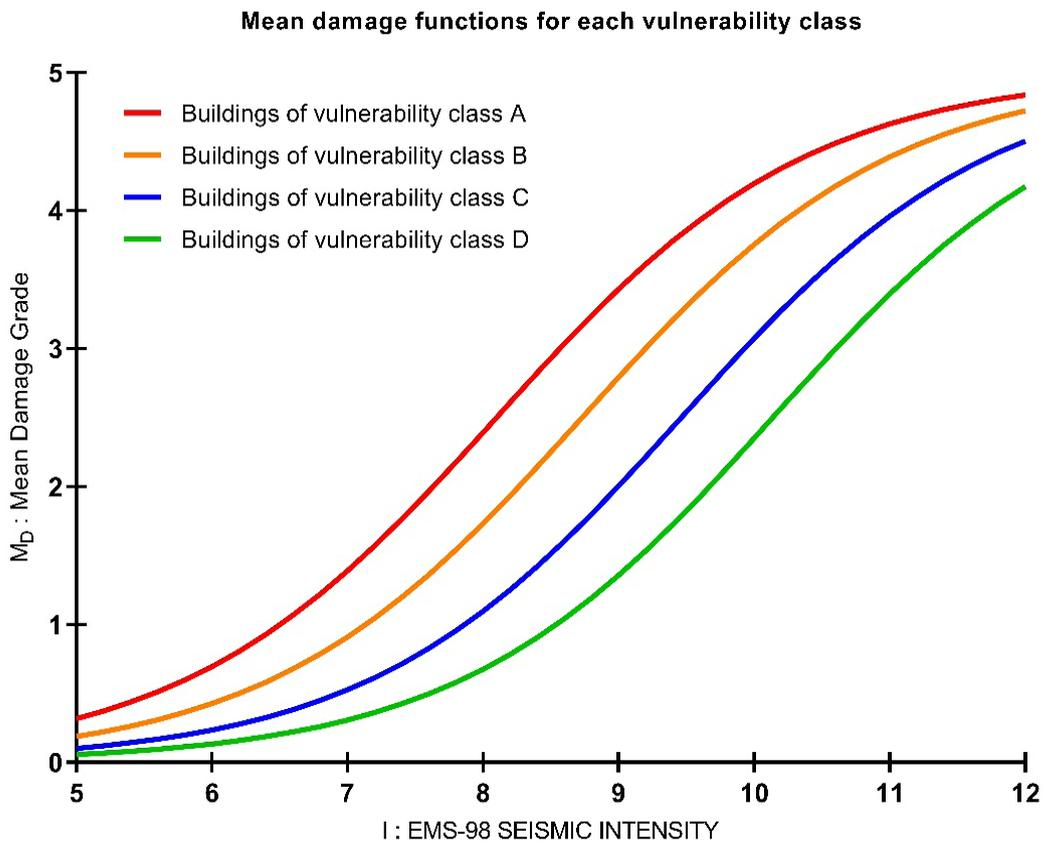
Figure 4. Mean damage functions for each vulnerability class in the urban area of Taza.
