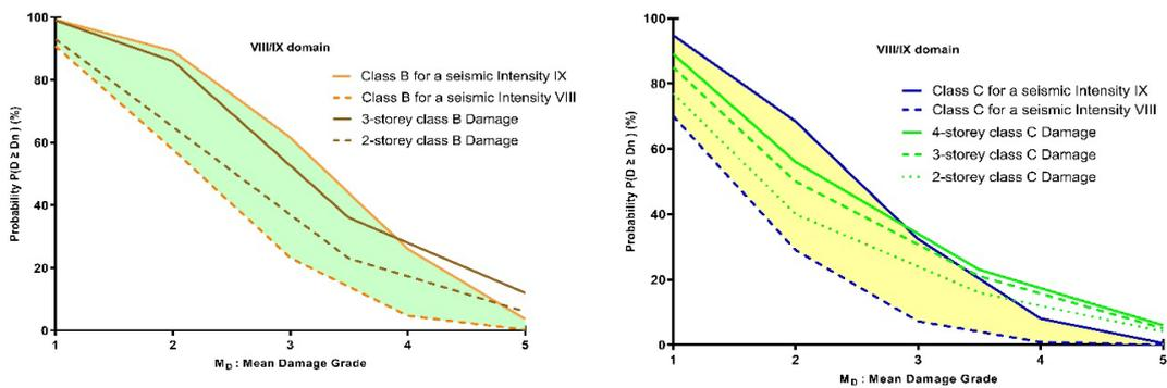
Figure 9. Comparison of damage percentages for vulnerability classes B and C.
