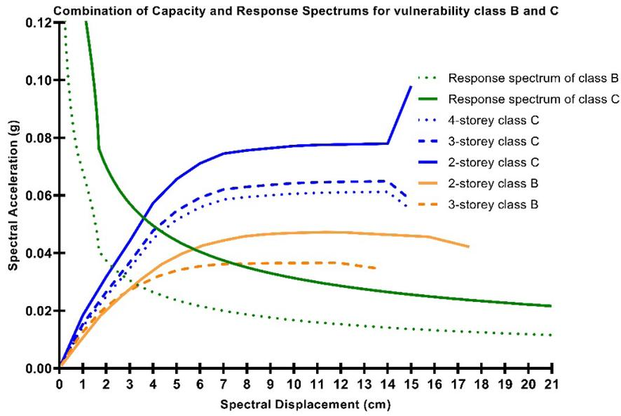
Figure 8a. Combination of capacity and response spectrums, identification of the performance point for the selected seismic classes B and C.
