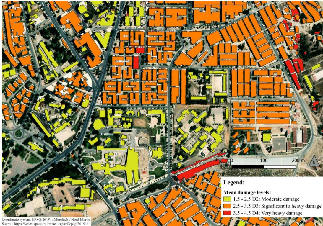
Figure 6. Distribution of mean damage levels for a seismic intensity scenario of IX in the Taza study area.
